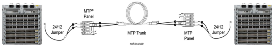
Figure 3: 100G Connectivity with Inter-Connect Structured Cabling
