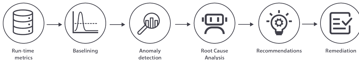
Figure 16: Proposed workflow of fully automated RCA engine
