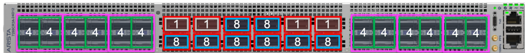
Figure 14d: 7280CR3A-24D12 default breakout capabilities (* indicates not all signaling lanes are used)
