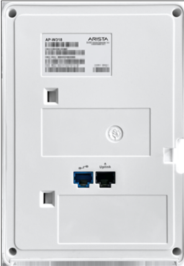
Figure 3-2: W-318/W-318 RW Rear Panel
