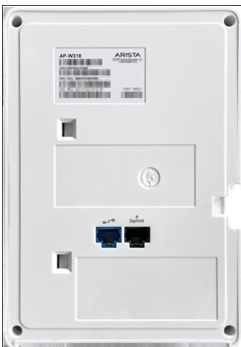
Figure 4-4: Back panel of the AP showing the network ports
